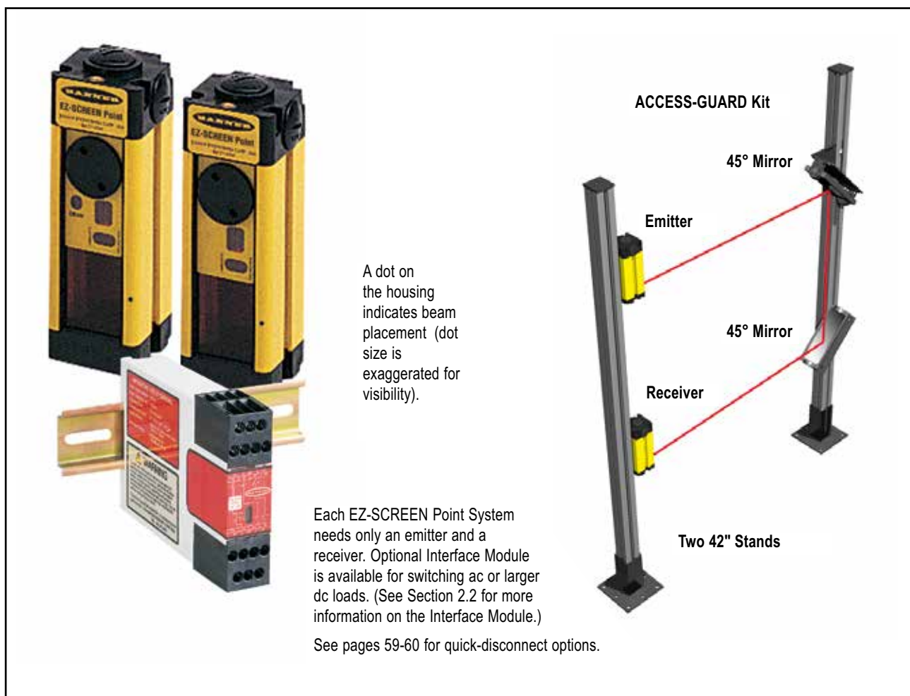
Figure 1-1. EZ-SCREEN Point components
