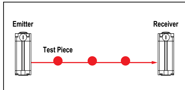
Figure 6-1. EZ-SCREEN Point trip test
