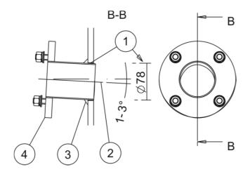
Counter flange which has been welded at correct angle to duct
