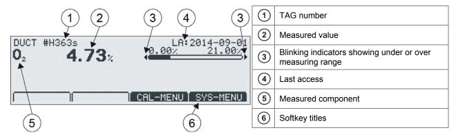
Figure 17 - Measuring mode
