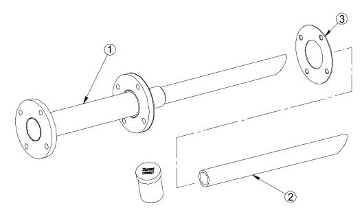
Figure 37 - Cooling tube components
