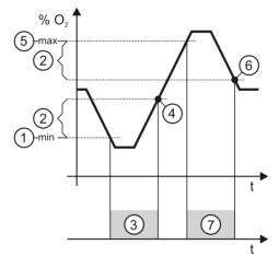
Figure 20 - O2 limit alarm settings
