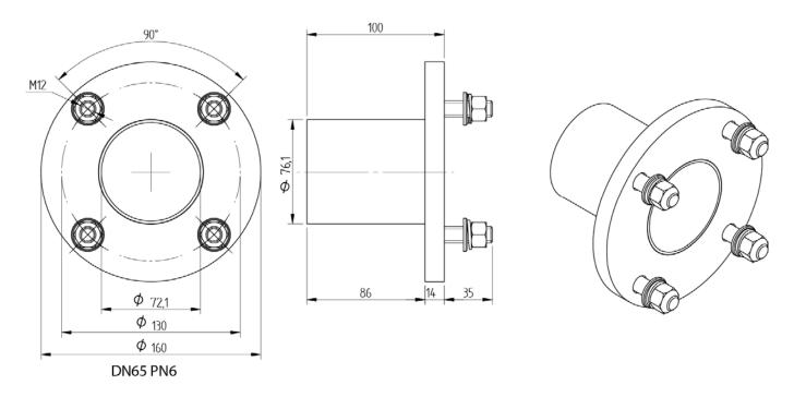
Figure 33 - Dimensions of counter flange
