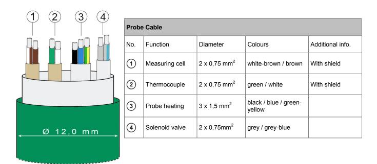
Figure 6 - Probe cable
