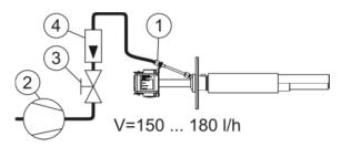
Figure 26 - Test air supply
