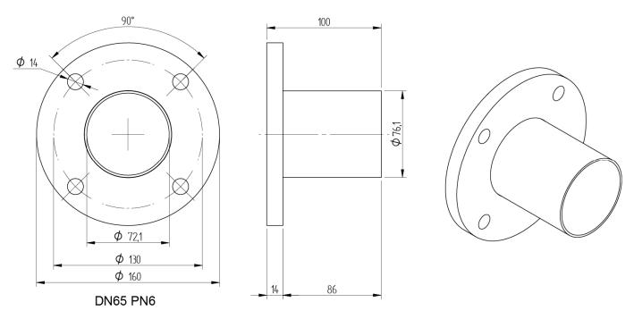
Figure 32 - Dimensions of counter flange
