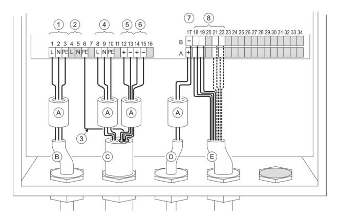
Figure 8 - Electrical connections of the electronic unit
