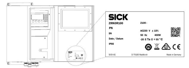
Figure 3 - Name Plate Electronic Unit
