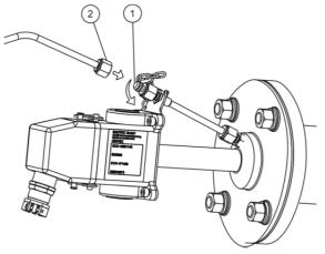
Figure 25 - Connect test gas tube
