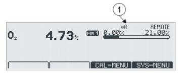
When a REMOTE connection to the analyzer is active, the connection is shown in the upper right corner of the display ①.
