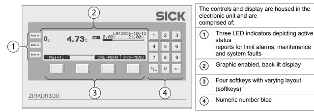
Figure 18 - Keypad and display
