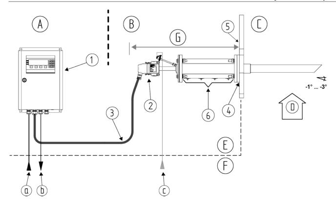
Figure 2 - ZIRKOR100 system (with cooling protection tube for flue gas temperatures of up to 1400°C)
