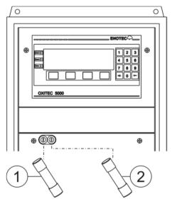
Figure 38 - Electronic unit - main fuses
