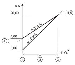
Figure 19 - O<sub>2</sub> Measuring Ranges
