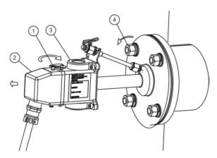
Figure 28 - O<sub>2</sub> probe dismounting
