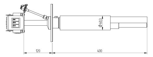
Figure 30 - High Dust Probe (max. 400°C)
