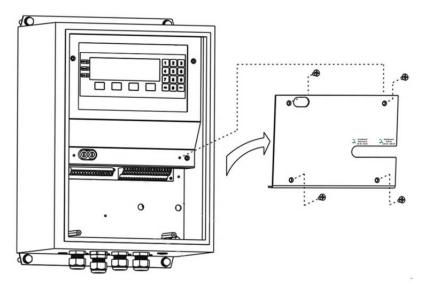
Figure 7 - Access to the terminals
