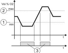
Figure 41 - O<sub>2</sub> Limit alarms
