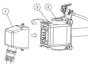
O<sub>2</sub> Probe plug 1 has to be inserted into the probe socket 2 and locked with the retaining clip 3.
