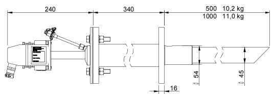
Figure 31 - Low Dust Probe (max. 1400°C)
