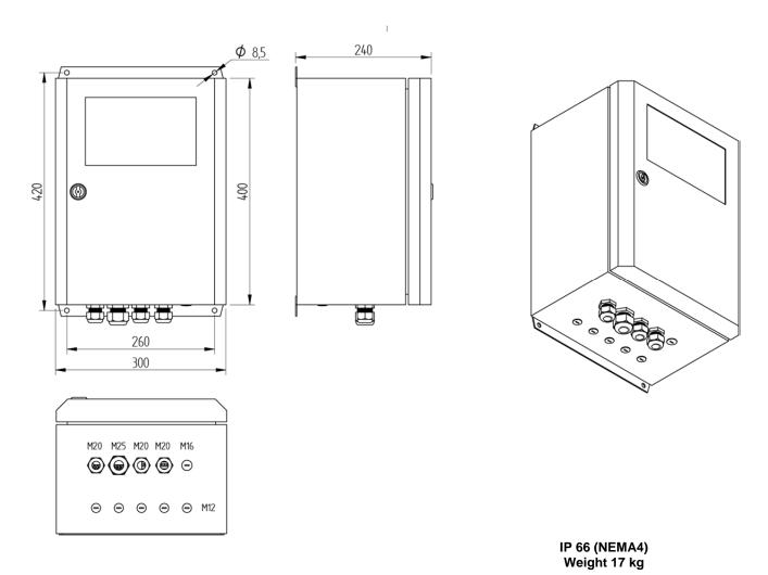
Figure 34 - Dimensions of electronic unit
