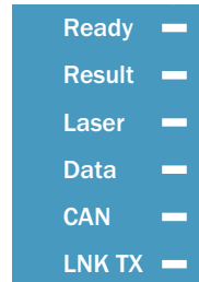
Figure 29: LED status indicator
