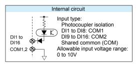
Note: Do not apply voltage outside the allowable input voltage range across input terminals. Doing so can cause a malfunction
