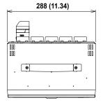
Unit: mm (approx. inch) Unless otherwise specified, tolerance is ±3% (however, tolerance is ±0.3 mm when below 10 mm).
