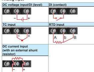
Be careful because the DI wiring is different between level and contact.
