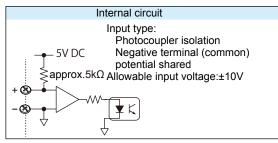
Note: Do not apply voltage outside the allowable input voltage range across input terminals. Doing so can cause a malfunction.
