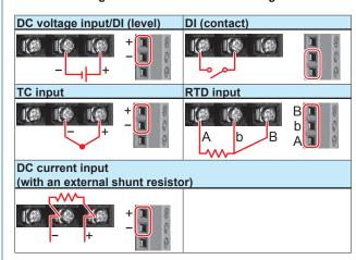
Be careful because the DI wiring is different between level and contact.
