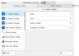
Tap the Quick setting tab. Setting menu of the quick setting is displayed.
