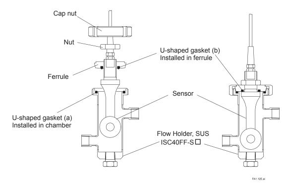
(a) (b) Gaskets in chamber and ferrule are recommended to be replaced with new ones (separately purchased) when sensor is replaced.
