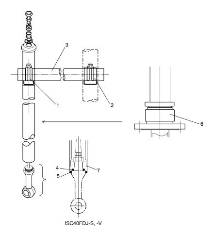
Qty Description Item Part No. Clamp (Option code: /MS1) Clamp (Option code: /MS2) Clamp (Option code: /MS1) Clamp (Option code: /MS2) Pipe (Option code: /MS1) L9813VP 1 1 2 1 L9813VP 2 L9813VN L9813VN K9144AM 3 Pipe (Option code: /MS2)
