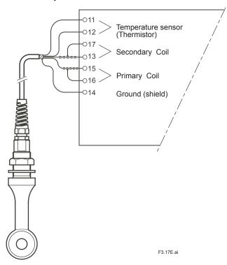
Figure 3.17 Wiring Diagram
