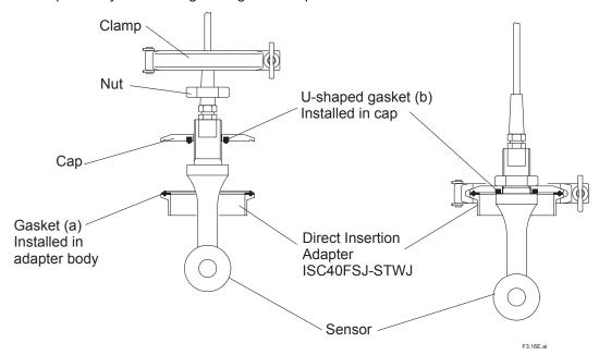
(a) (b) Gaskets in adapter and cap are recommended to be replaced with new ones (separately purchased) when sensor is replaced.
