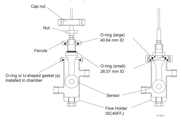
(a) O-ring or gasket in chamber is recommended to be replaced with new one (separately purchased) when sensor is replaced.
