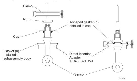
(a) (b) Gaskets in subassembly and cap are recommended to be replaced with new ones (separately purchased) when sensor is replaced.
