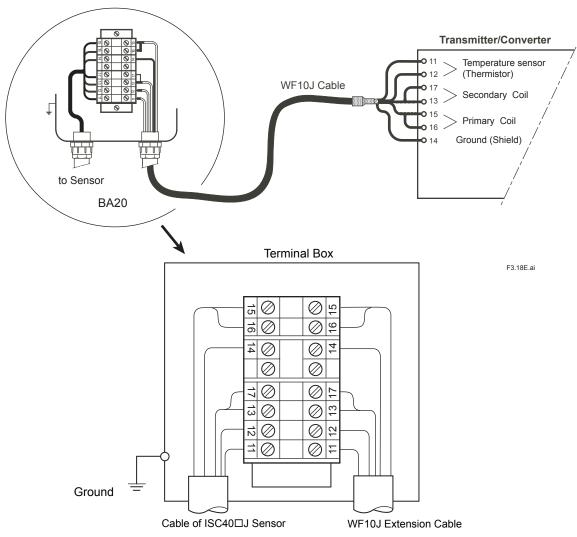
Figure 3.18 Connecting WF10J extension cable to BA20 terminal box
