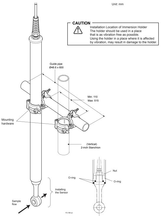
Figure 3.10 Method of Installing an Immersion Holder
