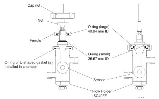
(a) O-ring or gasket in chamber is recommended to be replaced with new one (separately purchased) when sensor is replaced.
