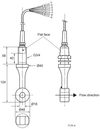
Figure 3.2 Installation of Sensor
