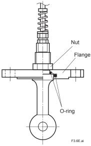
Figure 3.6 Direct flange mounting
