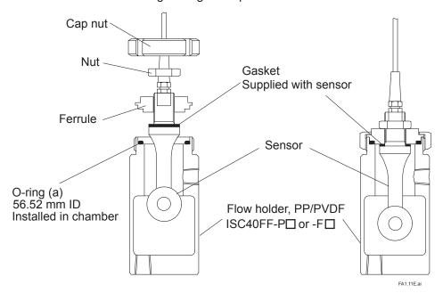
(a) O-ring in chamber is recommended to be replaced with new one (separately purchased) when sensor is replaced.
