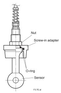
Figure 3.7 Optional screw-in adapter
