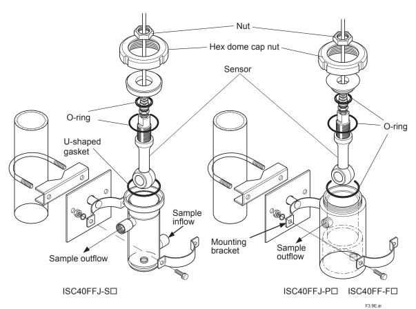
Figure 3.9 Example of Installing a Flow-through Holder
