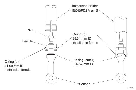
(a) (b) O-rings in ferrule are recommended to be replaced with new ones (separately purchased) when sensor is replaced.
