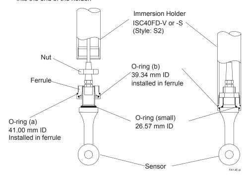
(a)(b) O-rings in ferrule are recommended to be replaced with new ones (separately purchased) when sensor is replaced.
