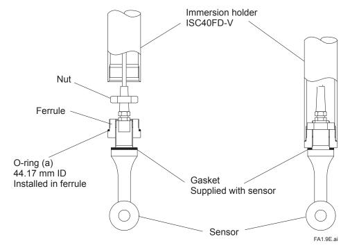
(a) O-ring in ferrule is recommended to be replaced with new one (separately purchased) when sensor is replaced.
