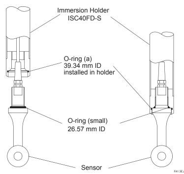
(a) O-ring in holder is recommended to be replaced with new one (separately purchased) when sensor is replaced.
