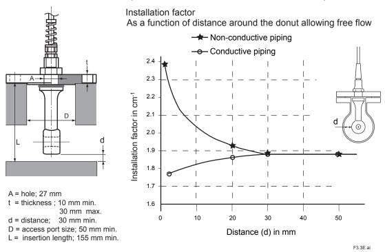
Figure 3.3 Example of Flange or Pipe Mounting, Installation Factor
