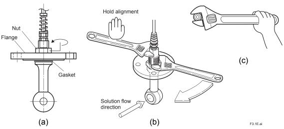
Figure 3.1 Sensor mounting
