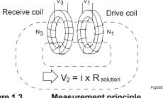
Figure 1.3 Measurement principle
