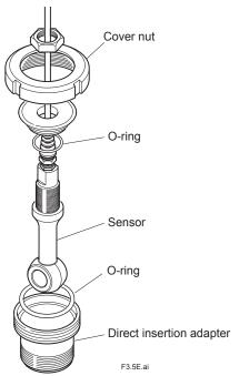
Figure 3.5 Installing Sensor with adapter
