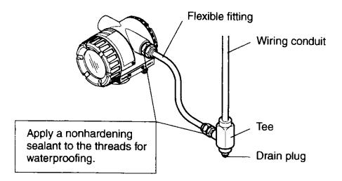
For Flameproof type, use Flameproof Packing Adapter or Flameproof Conduit in connection above.
