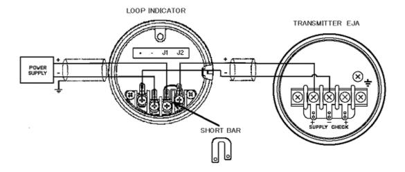
The Loop Indicator is available in FM Explosion Proof and CSA Explosion Proof types for hazardous locations. Wire sealing is required for these approvals. The following diagrams show some wire sealing examples.
