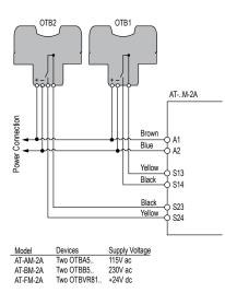
Figure 5. Type IIIA hookup to two OTB touch buttons with contact outputs
