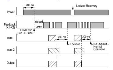
Figure 8. X1 and X2 Input timing requirements
