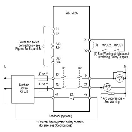
Figure 9. Machine control circuit connections
