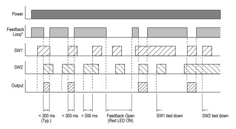
Figure 2. DUO-TOUCH Safety Module AT-..M-2A timing diagram
