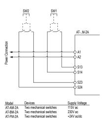
Figure 7. Type IIIB hookup to two mechanical push buttons with contact outputs
