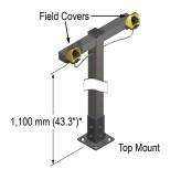
Figure 3. Install activation devices so that they are protected to prevent defeat or inadvertent actuation
