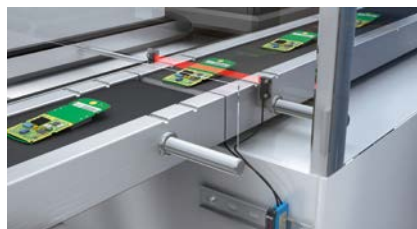
Leading edge detection for PCBs
