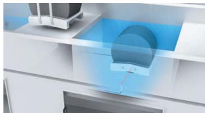
Wafer detection in wet process
