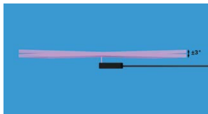
Safe detection of lead frames, even in a slanted position
