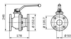
Ball valve, 3" version for standard temperatures
