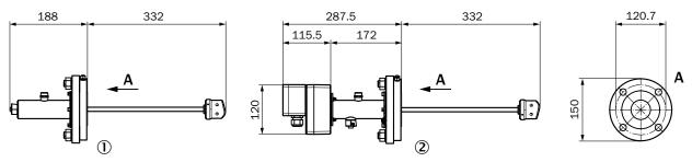
0 Sender/receiver unit (analog) for ATEX Ex zone 1, Ex zone 2, and CSA CI I, div 1/div 2
