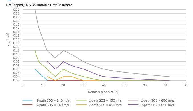
V<sub>min</sub> exemplary – 4" ... 16": EX-S with transducers for standard temperature range, 20" ... 72": EX-RE
