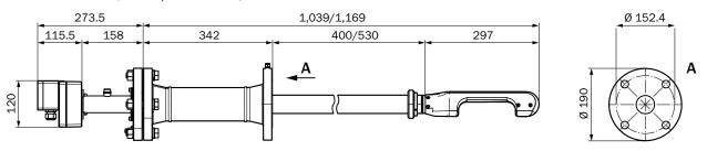
Sender/receiver unit (digital) with electronic unit for ATEX zone 2: Nominal length 400 mm for pipe diameters up to 48"; nominal length 530 mm for pipe diameters > 48" to 72"
