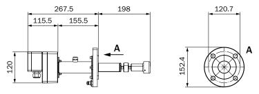
Sender/receiver unit (digital) with electronic unit for ATEX zone 2
