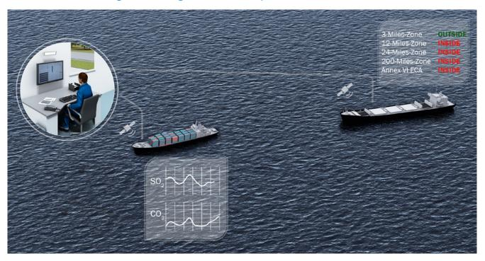
The MARSIC series of ship emissions measuring devices give ship operators the safety they need. In combination with the appropriate software, MARSIC generates an emissions profile that can be linked with the current ship location. This provides enormous added value: the ship's crew can initiate the necessary measures immediately on entering an Emission Control Area (ECA).
