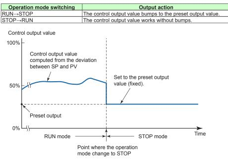
Preset output value is available for each PID parameter group and works according to the selected PID parameter group.
