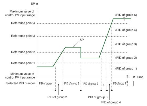
The control PV input range can be divided into the number of zones that is set in the reference point.
