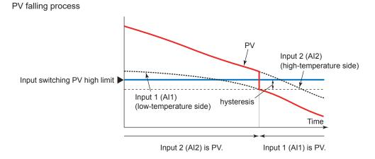
When input 1 (AI1) < input switching PV high limit – 0.5% of PV input range span, PV = input 1 (AI1) When input switching PV high limit – 0.5% of PV input range span  $\leq$  input 1 (AI1), PV =
