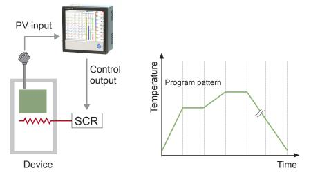
The program operation can be used to change the SP over time according to a preset program pattern.
