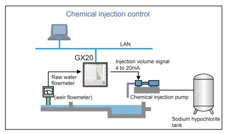
Injection volume of sodium hypochlorite is calculated based on the injection ratio, concentration, specific gravity in relation to the raw water flow rate. The injection volume setpoint is used to control or retransmit the setpoint to the pump.
