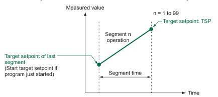
Set the segment time in the range of 00:00:01 to 99:59:59 (hour:minute:second). The segment time applies to all loops and is set for each segment.
