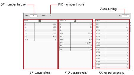
The SP number in use, PID number in use, and auto-tuning are displayed above the setting parameters. You can select the SP number and PID number with the list boxes. Parameters of the selected numbers are displayed. Double-clicking a parameter displays an edit dialog box.
