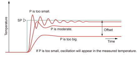
► For details on offset, see section 3.5.9, "Canceling the PV and SP Offset (Manual Reset)."
