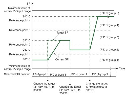
The control PV input range can be divided into the number of zones that is set in the reference point.
