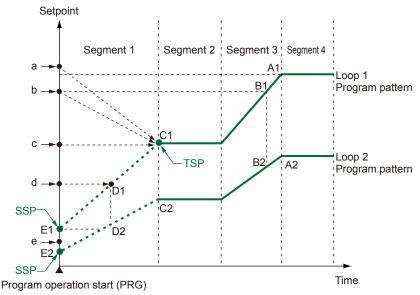
(The explanation below assumes that the reference loop is set to Loop-1.) When segments 1 and 2 of loop-1 program pattern are ramp and segment 3 is soak Program operation start point of Loop-1 is any of the points A1 to E1. Because the program pattern operation start point of Loop-2 is the same as that of Loop-1, if the program pattern operation start point of Loop-1 is A1, then that of Loop-2 is A2.
