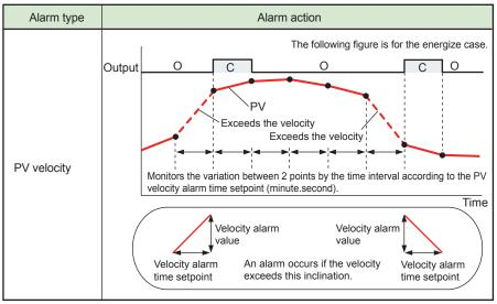
\* "O" and "C" indicate the relay contact open and close states.
