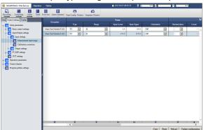
Set the PV input type, range, and span of loop number L091.
