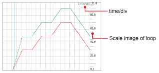
The area to the left of the pattern progress position cursor (past waveform area) shows PV and SP waveforms. The PV waveform is displayed only when recording.
