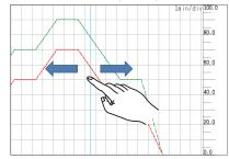
The area to the right of the pattern progress position cursor (future waveform area) shows pattern waveforms with broken lines.
