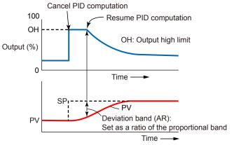
The parameter AR sets the point (by deviation band (%)) to restart the PID computation that is suspended by the controller's anti-reset windup function. PID computation restarts when the deviation band has decreased to the setpoint. When the anti-reset windup type is set to AUTO, the controller automatically determines the point at which to restart the PID computation.
