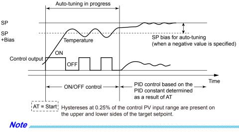
In time proportional output, the output is turned on and off irrespective of the upper/lower limit.
