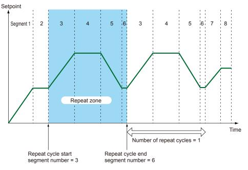
Is the start code is set to **Time-prioritized PV start** or **Ramp-prioritized PV start**, the start code setting is also applied to the start of repeat operation.
