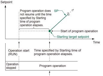
Operates according to the start code setting. The figure above is an example when the start code is set to starting target setpoint.
