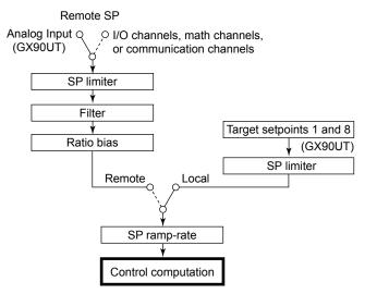
If the RSP input is an I/O channel, math channel, or communication channel, the GX/GP/ GM sends the most recent value of the specified channel to the PID control modules at the following transmission interval.
