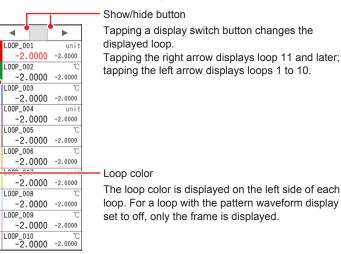
The maximum number of loops that can be displayed simultaneously in the loop area is 10. If there are more than 10 loops, you can switch the display using the display switch button. The layout in the loop area changes according to the number of loops assigned to the patterns.
