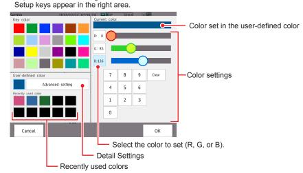
**3** Select R, G, B one at a time, and set each value using the numeric keypad or the bars.
