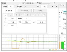
**4** Tap the **SP group** tab and then an alarm setpoint (A1, A2, A3, or A4). Parameter edit buttons appear.
