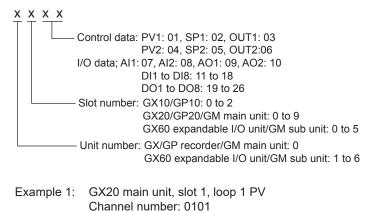
Example 2: GM10 sub unit 1, slot 4, slot 4 DO1 Channel number: 1419
