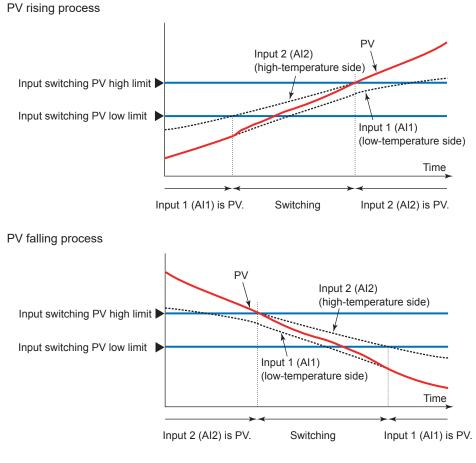
When input 2 (Al2) ≤ input switching PV low limit, PV = Input 1 (Al1)
