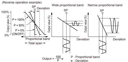
To fine-tune a proportional band obtained using auto-tuning, or to manually tune the proportional band:
