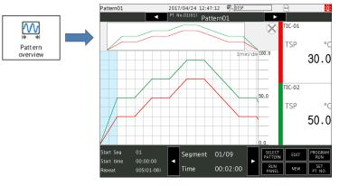
You can change the pattern position to display in the waveform area by tapping the overview area.
