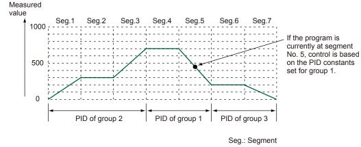
Zone PID selection (PV), Zone PID selection (target SP), External selection
