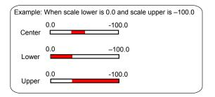
When Displaying the Current Value on the Scale Using the Bar Graph
