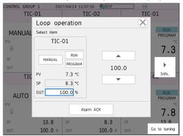
If the loop operation dialog box is opened from a program screen, the following buttons are also displayed.
