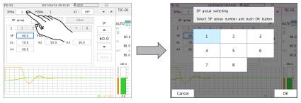
In case the PID selection is SP No. selection, in the SP group number switch dialog box, you can change the SP group number to use for control. PID group numbers are set in pairs with the SP group numbers.
