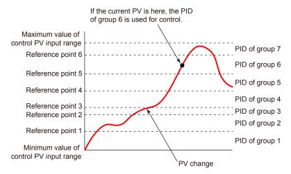
The control PV input range can be divided into the number of zones that is set in the reference point.
