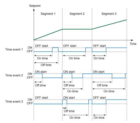
Time event action when start code (STC) is set to ramp-prioritized PV start When operation is started in the middle of a segment by the start code (STC), the event action starts in the event setting state at the time when operation should have started, on the assumption that the set event action has been performed by that time.
