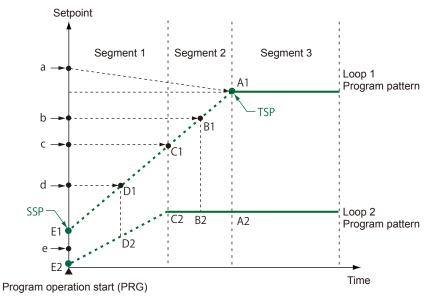
If the Program Pattern of Loop-1 Does Not Contain Soaking (The explanation below assumes that the reference loop is set to Loop-1.) Program operation start point of Loop-1 is any of the points A1 to E1. Depending on the PV, the program advances to segment 5. If the PV is point a, the program advances until point A1, where the ramp-rate is inverted.
