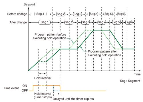
Hold operation is also released by advancing the segment or by running or resetting to the program operation.
