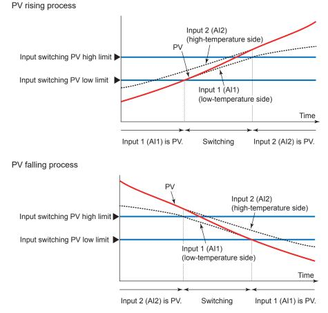
When input 1 (AI1) ≤ input switching PV low limit, PV = Input 1 (AI1)
