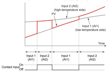
Control output will change smoothly (i.e., without any bumps) when PV switches.
