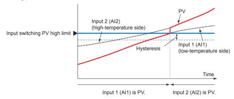
When input 1 (AI1) < input switching PV high limit, PV = Input 1 (AI1) When input switching PV high limit  $\leq$  input 1 (AI1), PV = Input 2 (AI2)
