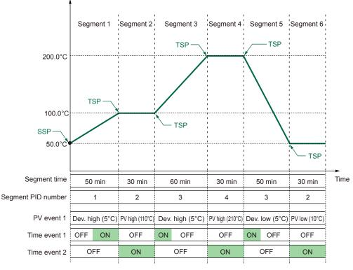
SSP: Starting target setpoint TSP: Target setpoint
