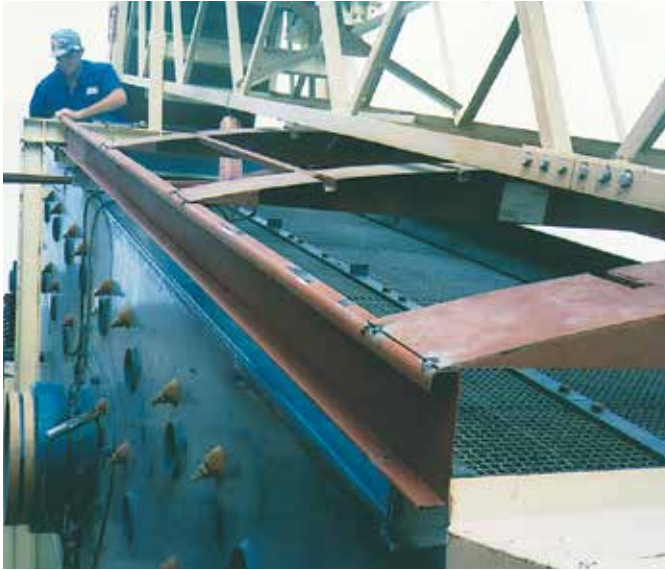
Trellex 300TS with flexible rubber prevents blinding
