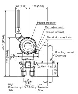
Measurement span code F or option code /HD, /HD2
