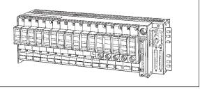
Withstand voltage: 1500 V AC/min. between input and (output and power supply.) 500 V AC/min. between output and power supply.
