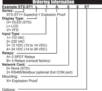
ET= Extended Temperature LCD Display -4°F to 131°F (-20°C to 55°C)
