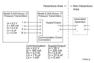
Note: The Associated Apparatus must be a linear power source.
