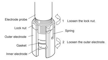
Figure 5.3 Removing the Outer Electrode and Lock Nut
