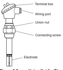
Figure 3.5 Union Nut for Direction Adjustment of Terminal Box
