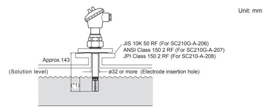
\*1: Always keep the electrode tip dipped more than 60 mm for SC210G-A, more than 100 mm for SC210G-B.
