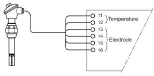
SC210G Conductivity Detector (two-electrode system) Applicable Analyzer: FLXA402, SC450G, FLXA202, FLXA21
