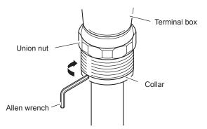
Figure 5.4 How to Remove Electrode Assembly
