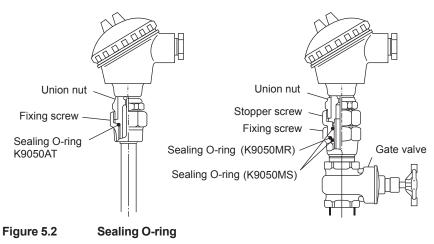
For the direct insertion type conductivity detector with gate valve, proceed as follows for inspection and replacement.
