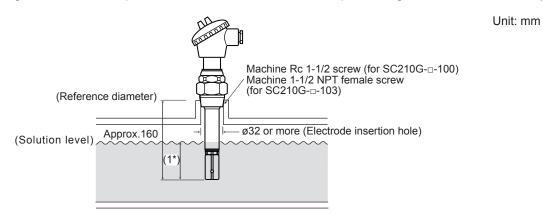
\*1: Always keep the electrode tip dipped more than 60 mm for SC210G-A, more than 100 mm for SC210G-B.
