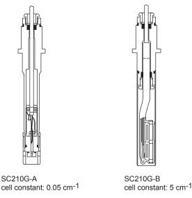
Figure 1.1 Electrode Construction of the Conductivity Detectors
