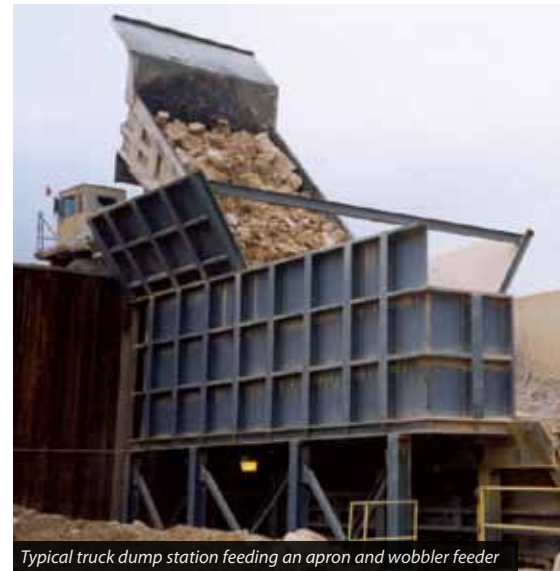
Typical truck dump station feeding an apron and wobbler feeder
