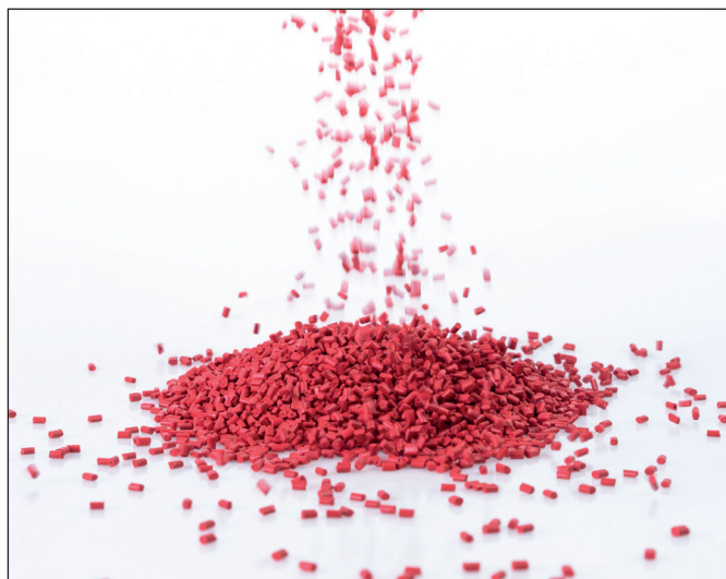
Fig. 2: Plastic granulate for injection molding or extrusion
