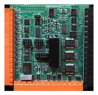
Figure 8.2 - XL7 I/O Cover Removed (sample I/O board)
