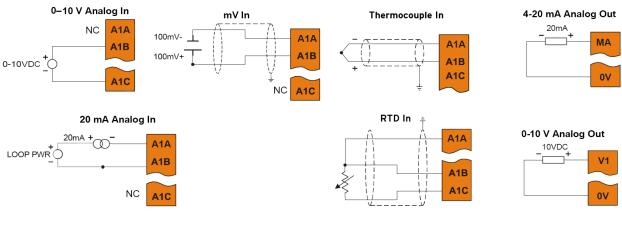
**NOTE:** Depending on the transmitter, isolated loop power may be required.
