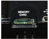
Figure 17.1 - Removable microSD Memory Card Slot
