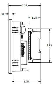
Figure 3.5 - Extended I/O Back Cover Dimensions
