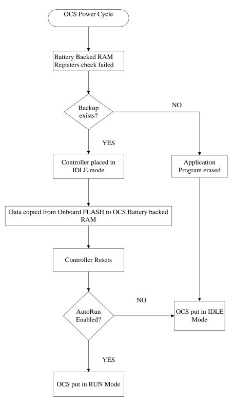
Figure 19.6 - Flow Chart for Automatic Restore
