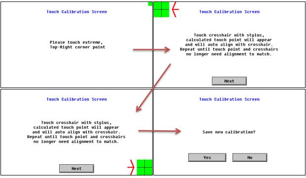
Figure 5.3–Screen Calibration
