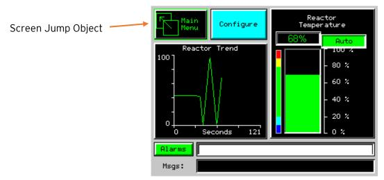
Figure 14.3 - Typical Screen Jump Object
