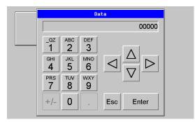
In addition, to edit a single numeric digit, use the  $\leftarrow$  or  $\rightarrow$  key to select the digit and then either press a numeric key or use  $\downarrow$  or  $\uparrow$  to modify the digit. In any case, after entering the new desired value, press the **Enter** key to save it; otherwise press the **ESC** key to cancel the edit.
