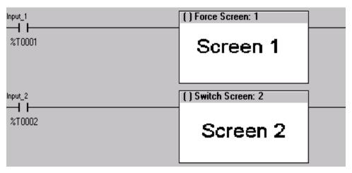
Figure 14.4 - Force and Switch Coils in Ladder Programming
