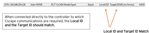
If the controller is not communicating, ensure the target ID is set correctly. If not, set the target ID of the controller in Cscape or on the unit. The **Target ID** allows directing communications to a particular unit when multiple units are connected via a CsCAN network. Units without CsCAN network ports respond to any network ID and do <u>not</u> require the ID to be configured.
