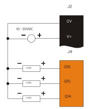
Figure 8.4 - Typical Output Wiring
