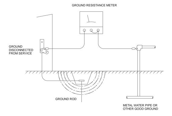
Figure 4.1 - Two-Point Ground Connection Test
