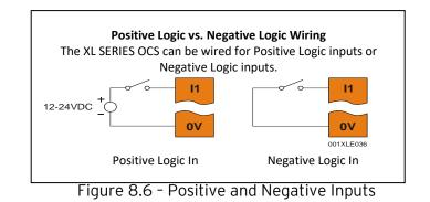
In positive logic mode a positive voltage applied to the input will turn the input. The internal design of this mode is basically a resistor from the input to I/O ground. This mode is sometimes called "sourcing".
