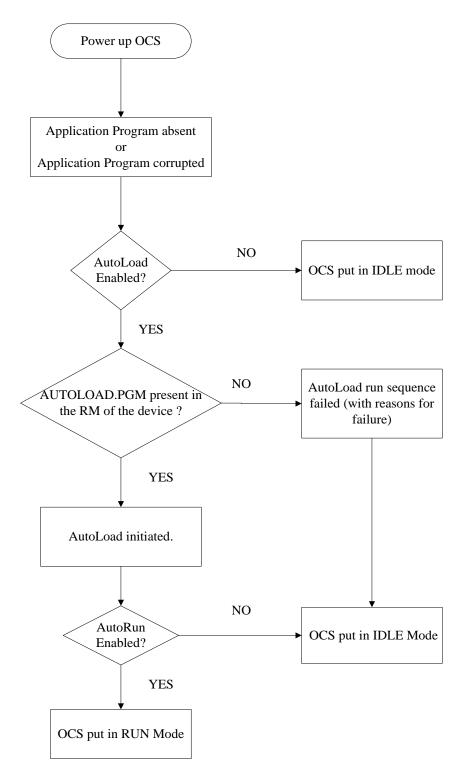
Figure 19.8 - Flow Chart for AutoLoad
