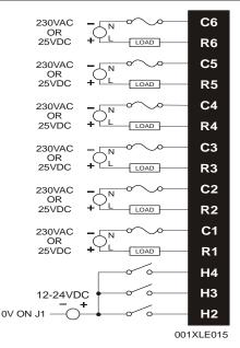
Figure 8.5 – Relay Fusing
