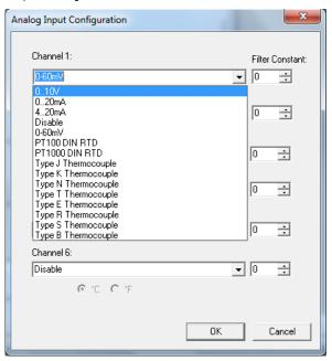
Figure 8.8 - Analog Input Configuration Screen
