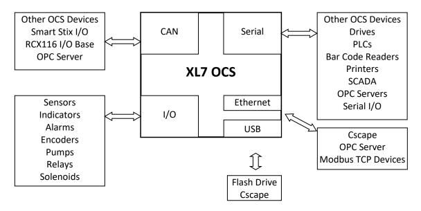
Figure 2.2 - Visual Overview of Types of Devices that can be connected to XL7 OCS
