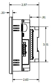
Figure 3.4 - Standard Back Cover Dimensions
