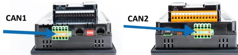
Figure 11.1 - CAN1 & CAN2 Connector Locations
