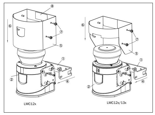
Fig. 6: Mounting with VdS mounting kit
