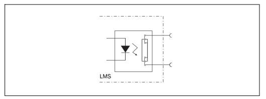
Fig. 10: The fault output with optocoupler
