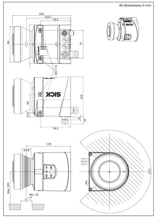
Fig. 22: Dimensional drawing LMS/LMC12x
