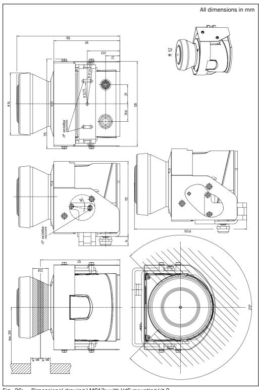
Fig. 26: Dimensional drawing LMC13x with VdS mounting kit 2
