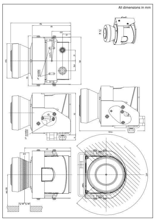
Fig. 25: Dimensional drawing LMC12x with VdS mounting kit 2
