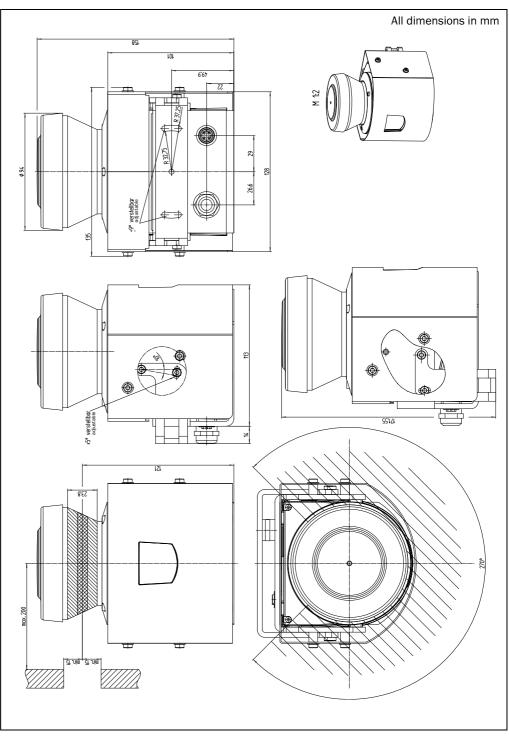
Fig. 24: Dimensional drawing LMC12x with VdS mounting kit 1
