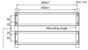
Supplied spacer(50) or Wiring space(30 to 60)
