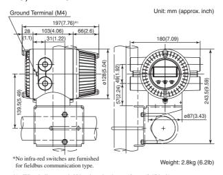
\*1: When indicator code N is selected, subtract 12 mm (0.47 inch) from the value in the figure. In case of explosion proof type with indicator, add 5 mm (0.2 inch) to it.  $_{\sf F06.EPS}$
