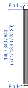
Extension cable molex to molex 140 mm: Part no. 254 642-1 340 mm: Part no. 254 642-2 640 mm: Part no. 254 642-3
