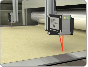
L-GAGE® LH Series Laser Sensors deployed on the sprout line measure dough height prior to baking
