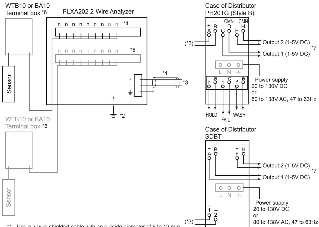
\*1: Use a 2-wire shielded cable with an outside diameter of 6 to 12 mm.
