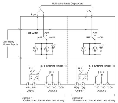
(1) When shipped from the factory, output 1 a / b switching jumper is set to a-contact.
