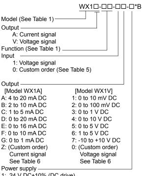
1: 24 V DC±10% (DC drive) 2: 85 to 264 V AC (AC drive)
