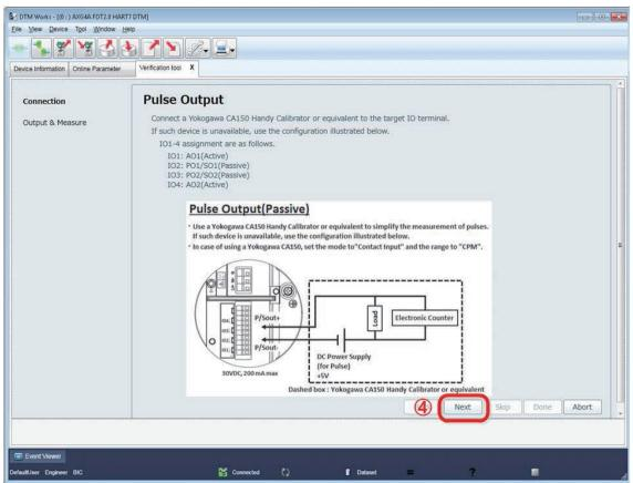
Figure 7.2.17 Wiring for Pulse Output Check
