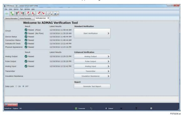
Figure 7.2.30 Finishing Analog Input Check
