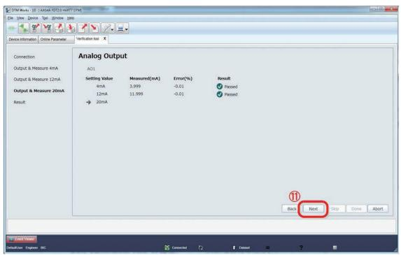
Figure 7.2.11 Continuing Analog Output Check
