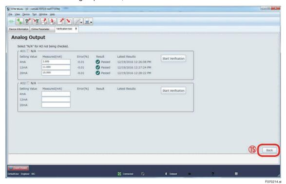
Figure 7.2.14 Finishing Analog Output Check
