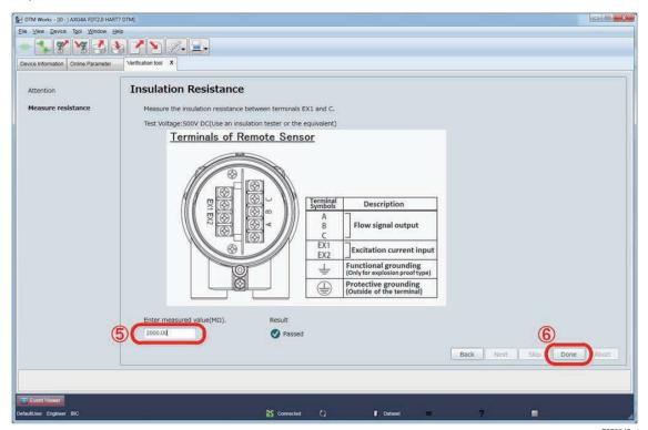
Figure 7.2.45 Measuring Insulation Resistance
