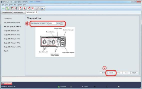
Figure 7.2.35 Setting Span Setting Dial of AM012 Calibrator
