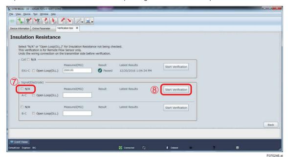
Figure 7.2.46 Continuing Insulation Resistance Check
