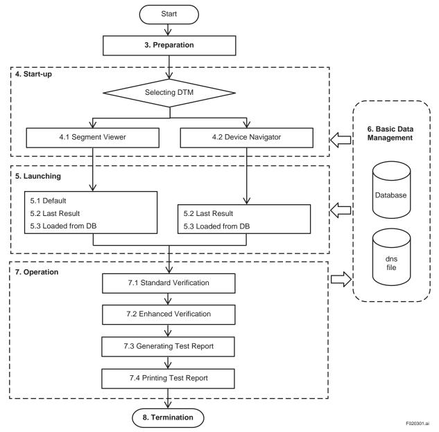
Figure 2.3.1 Operation Procedure
