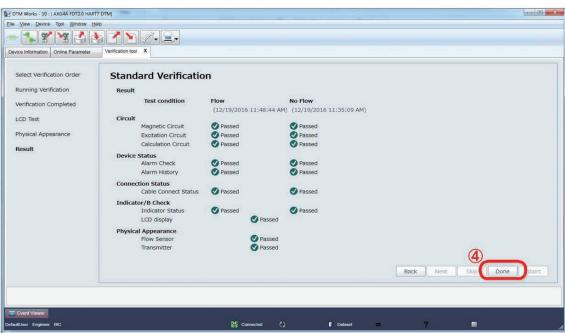
Figure 7.1.12 Result of Standard VF
