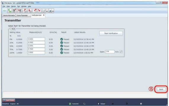
Figure 7.2.41 Finishing Transmitter Check
