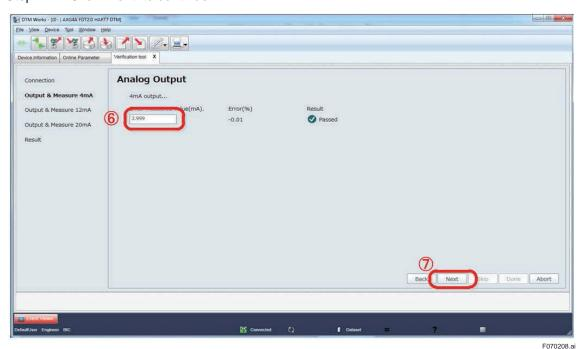
Figure 7.2.8 Entering Measured Analog Output Value
