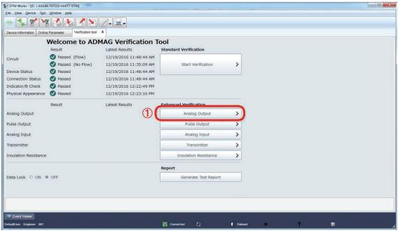
Figure 7.2.4 Selecting Analog Output Check
