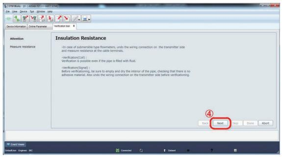
Figure 7.2.44 Continuing Insulation Resistance Check
