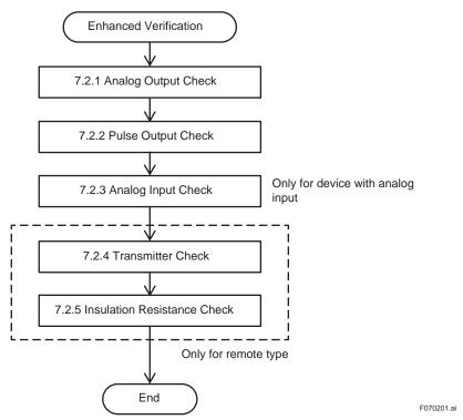
Figure 7.2.1 Procedure of Enhanced VF
