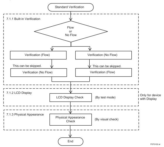
Figure 7.1.2 Procedure of Standard Verification
