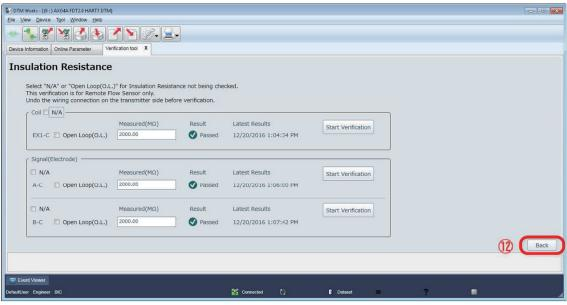
Figure 7.2.49 Finishing Insulation Resistance Check
