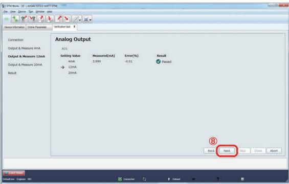
Figure 7.2.9 Continuing Analog Output Check
