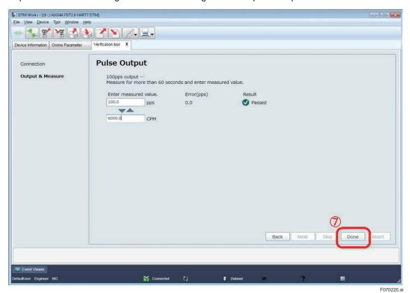
Figure 7.2.20 Continuing Pulse Output Check
