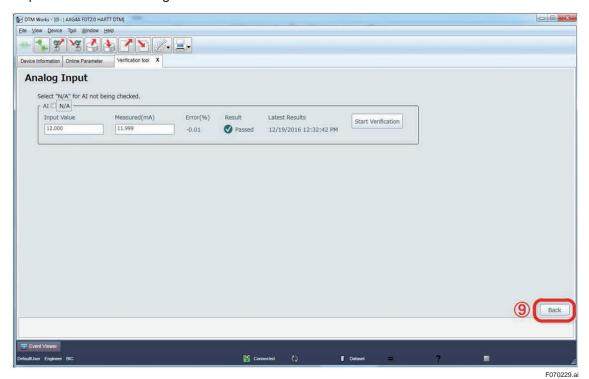
Figure 7.2.29 Finishing Analog Input Check
