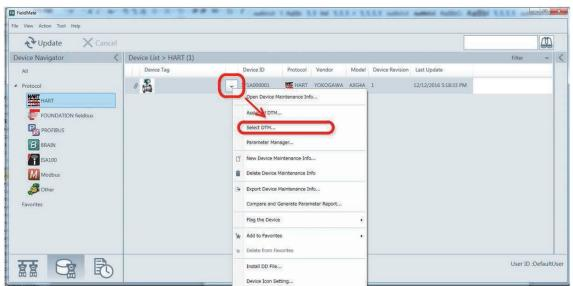
Figure 4.2.2 Starting Up DTM by Device List
