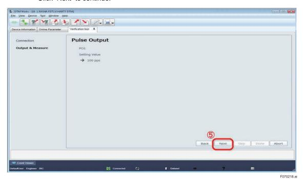
Figure 7.2.18 Continuing Pulse Output Check
