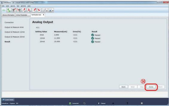
Figure 7.2.13 Continuing Analog Output Check
