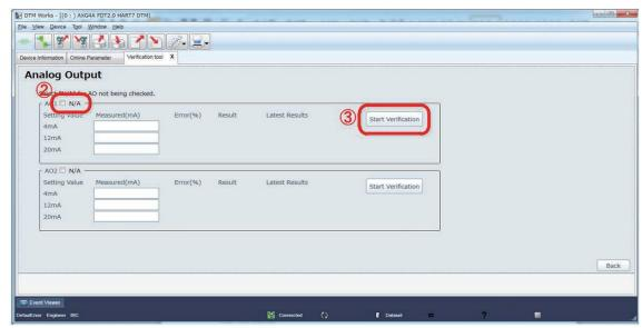
Figure 7.2.5 Starting Analog Output Check
