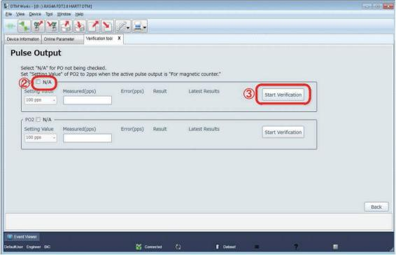
Figure 7.2.16 Starting Pulse Output Check
