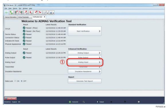
Figure 7.2.22 Selecting Analog Input Check
