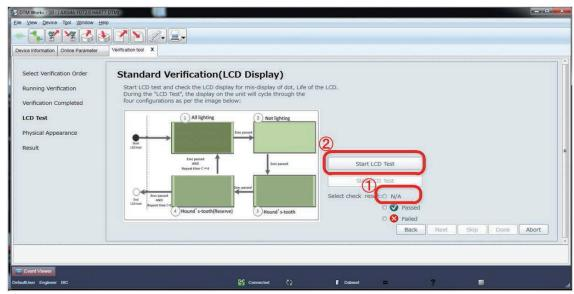
Figure 7.1.9 Starting LCD Display Check
