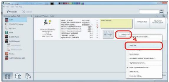
Figure 4.1.3 Starting Up DTM by Action Button
