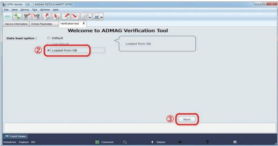
Figure 5.1.4 Selecting "Loaded from DB"
