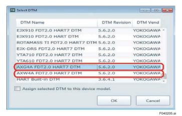
Figure 4.2.5 Selecting Target DTM
