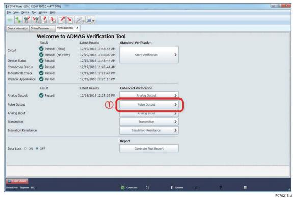
Figure 7.2.15 Selecting Pulse Output Check
