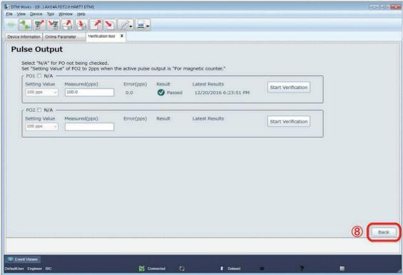
Figure 7.2.21 Finishing Pulse Output Check
