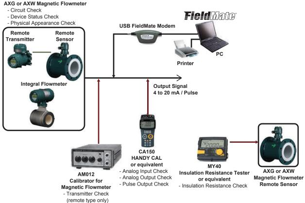
Figure 2.1.1 System Configuration
