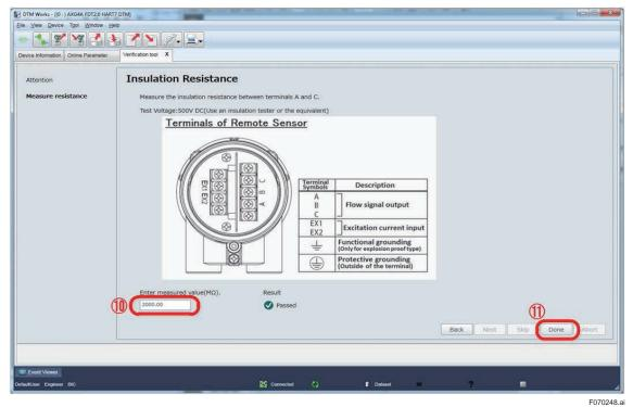
Figure 7.2.48 Continuing Insulation Resistance Check
