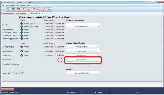
Figure 7.2.31 Selecting Transmitter Check
