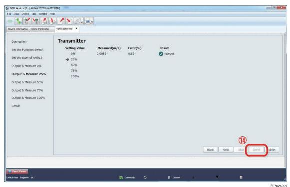
Figure 7.2.40 Continuing Transmitter Check
