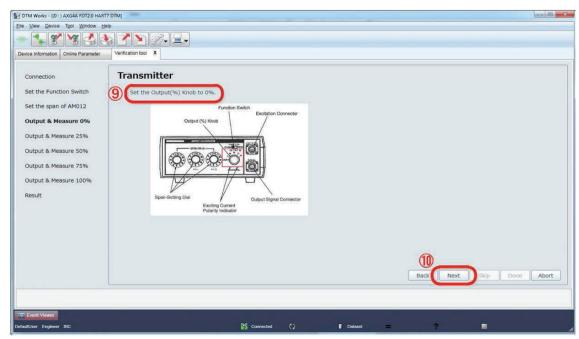
Figure 7.2.37 Setting Output Dial of AM012 Calibrator
