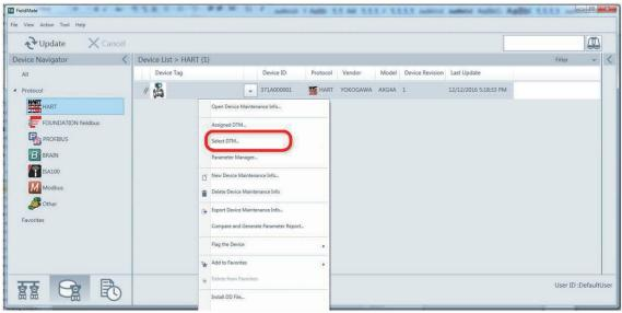
Figure 4.2.4 Starting Up DTM by Right-clicking
