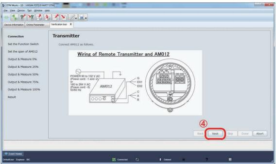
Figure 7.2.33 Wiring for Transmitter Check
