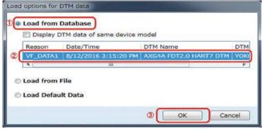
Figure 6.2.1 Loading during Starting Up DTM
