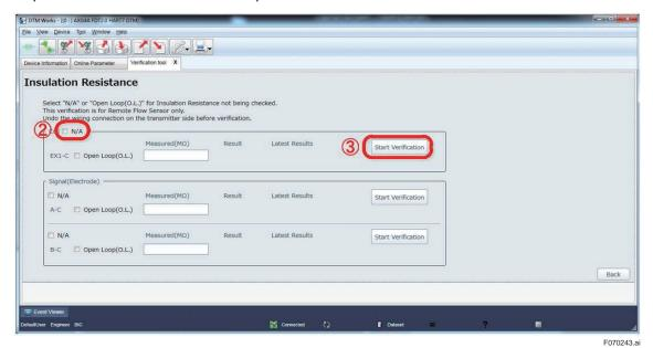
Figure 7.2.43 Starting Insulation Resistance Check
