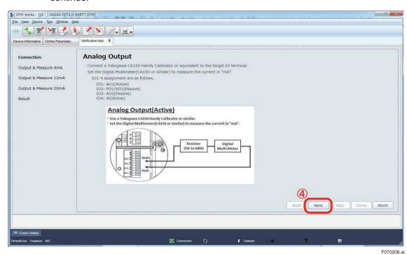
Figure 7.2.6 Wiring for Analog Output Check
