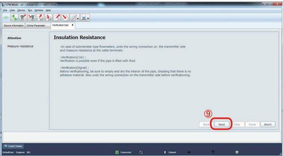
Figure 7.2.47 Continuing Insulation Resistance Check
