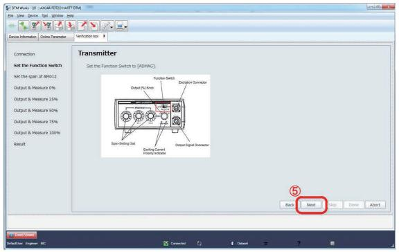
Figure 7.2.34 Setting Function Switch of AM012 Calibrator
