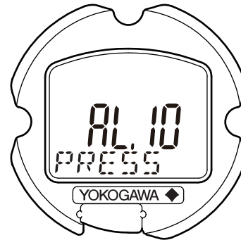
Self-diagnostic error on integral indicator (Faulty transmitter)
