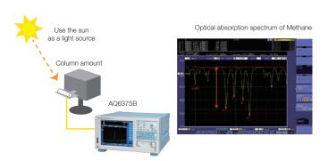
Figure 5 – Measurement setup to detect a specific gas in the air, e.g. Methane (CH<sub>a</sub>) with AQ6375B
