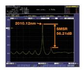
Figure 1 – Measurement example of 2010 nm DFB-LD with AQ6375B (Res: 0.05 nm, Span: 20 nm)
