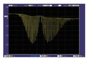
Figure 4 – Hydrogen Cyanide  $H_{13}C_{14}N$  absorption spectrum measurement with AO6375B
