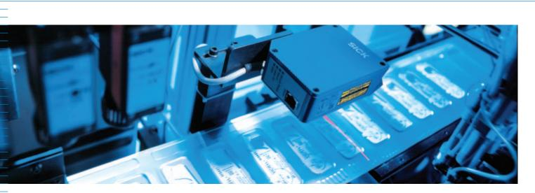
When fix-mounted scanners are used for barcode identification, it is also important to consider whether or not the object to be identified is moved:
