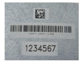
interpretation the code is. In theory, the amount of data a linear code can contain is unlimited. In practice, however, it is extremely limited because the code requires sufficient space in the reader's reading window and on the object itself.
