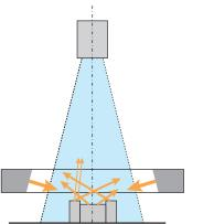
The light source is aligned in relation to the camera in such a way that the majority of the reflected light is not parallel to the optical axis of the camera. Only light that reflects on the edges runs parallel and thereby falls on the image sensor of the camera. As a result, the edges of the object are illuminated while the background remains dark. The dark field illumination method is particularly well suited to dot peening.
