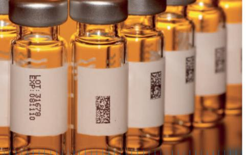
Unlike OCR, OCV (Optical Character Verification) does not read a text string, but instead compares a previously taught-in text with the text found on the object. This takes place via image processing algorithms that, for example, determine the total number of pixels or recognize the contours. The result of OCV is, therefore, either a "TRUE" or a "FALSE" with a supplementary evaluation of the correctness, quality, and readability of the string.
