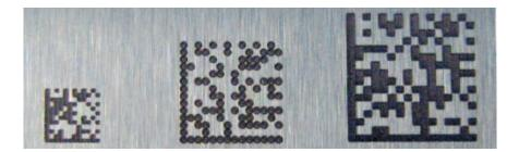
The dots should deviate as little as possible from the theoretical reference grid, that is, the ideal dot position or dot center. A deviation is referred to as a **dot center offset**.
