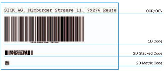
The data content and bar width or dot size is identical in all codes.
