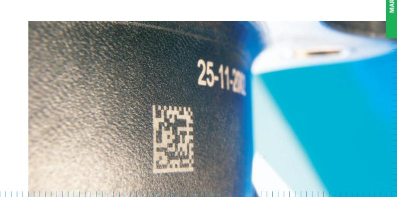
As defined in AS 9132, the following rule of thumb applies: The data matrix code should span a maximum distance of 16% of the diameter or 5% of the circumference of the cylindrical body. Rectangular codes are better suited to curved surfaces because their data content is the same but with a reduced height. Stretching the code along the axis of the cylindrical body does not
