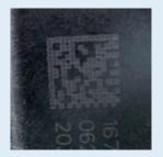
Laser type: CO<sub>2</sub> Object: Plastic Code quality: Readable code despite poor contrast between dots and background. **TIP:** Readability can be increased by changing the marking param-
