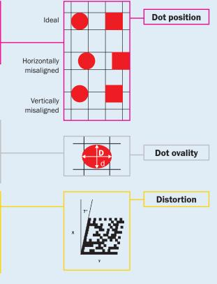
Depending on the marking method, it may only be possible to create round dots. Threshold values also exist for deviations from the ideal circle to ensure that the code can be read reliably. The difference between D and d should not exceed 20% of the dot size.
