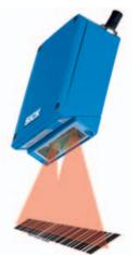
Two laser diodes illuminate a narrow section of a moving object. This illuminated section is captured by the line scan camera. The images that are captured line by line are reassembled as a whole, two-dimensional image by software algorithms in the reader. This image is then scanned for code structures after which the codes are decoded.
