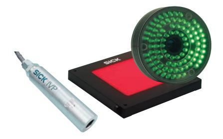
The reflectance behavior of the object surface and the spectral sensitivity of the camera chip determine the appropriate color. Red or white lighting is often used for code reading. The advantage of white light is that it is reflected by all object colors because it is comprises the entire visible color spectrum.
