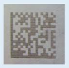
Object: Metal Code quality: Very good contrast between code and background, dots are square in form and completely filled (100%).
