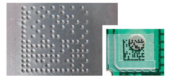
Dot peening on steel and ink jet printing on plastic
