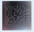
Object: Metal Code quality: Dot geometry, position, and degree of fill near ideal. **TIP:** Enlarge the quiet zone to the neighboring digit and reduce distortion to achieve a perfect code.
