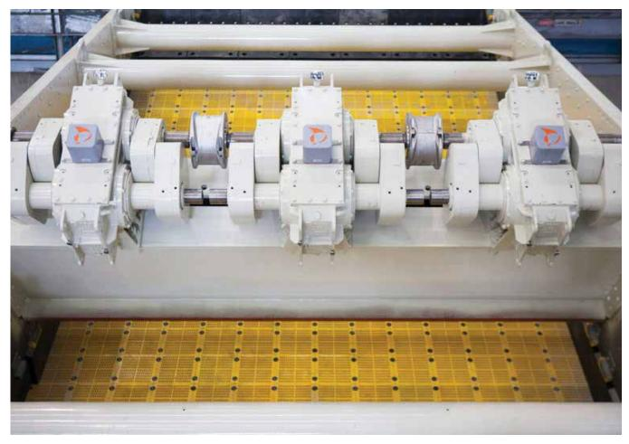
ScreenWatch monitors housing temperature and bearing wear in order to warn you of any potential bearing problems.
