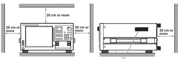
Also be sure to maintain sufficient clearance for connecting measurement cables.
