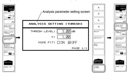
If you only want to change the THRESH LEVEL, you can also do so with the SPEC WIDTH THRESH soft key.
