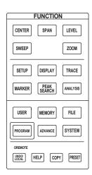
The FUNCTION section contains 17 function keys and 4 auxiliary keys. When you press a function key, information about the function is displayed on the soft key menu located on the right side of the LCD display.
