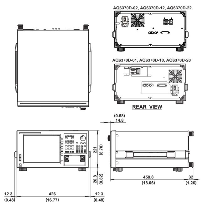
If not specified, the tolerance is  $\pm 3\%$ . However, in cases of less than 10 mm, the tolerance is  $\pm 0.3$  mm.
