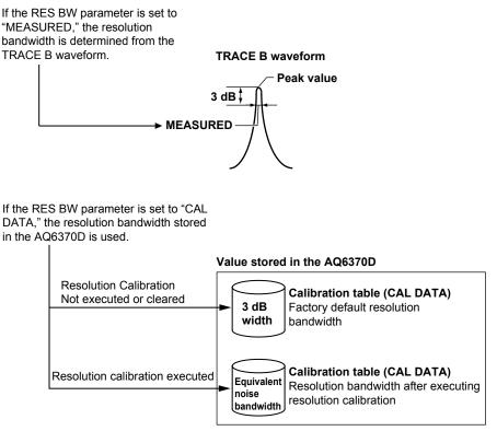
The analysis algorithm other than EDFA-NF uses the value stored in the AQ6370D.
