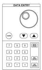
This unit allows you to enter measurement conditions and various other parameters through the DATA ENTRY section. Three different entry methods can be used in the DATA ENTRY section, the rotary knob, the arrow keys, and the numeric keypad.
