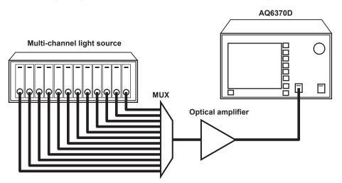
Measure the WDM signal light and write the waveform to the active trace.
