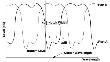
Obtain the width (xdB\_Notch\_Width) between the two points, which are above the bottom level of each channel by the parameter THRESH\_LEVEL, and its center wavelength (Center\_Wavelength).
