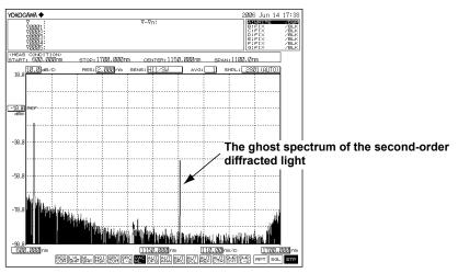
Example of measurement in which second-order diffracted light appears at 1266 nm
