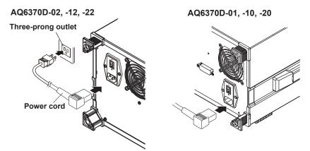
2. Turn ON the **MAIN POWER** switch on the rear panel of the instrument. The **POWER** switch on the front panel of the instrument lights orange.
