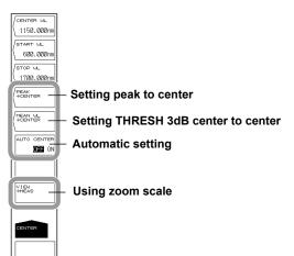
Also, you can set the wavelength of the moving marker placed on the measured waveform as the center wavelength or center frequency.
