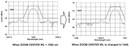
When ZOOM CENTER WL is changed to 1548.5 nm (template also moves in synch with the waveform)
