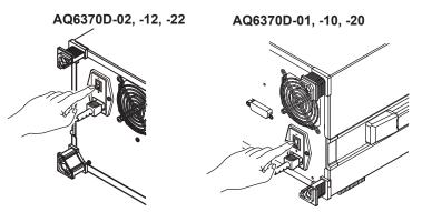
**3.** Press the **POWER** switch on the front panel of the instrument. The color of the switch turns from orange to green. The operating system starts up, and initialization of the instrument begins.
