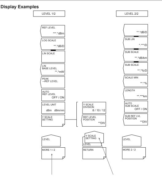
The LEVEL soft key menu is split into two parts. This key switches between the menus. In addition, in some cases this may change to a function that closes the window. For example, when the MORE 1/2 soft key is pressed, the menu changes to the LEVEL 2/2 soft key menu, and the key display changes to MORE 2/2. Shows the submenu of the soft key menu. In this example, the soft key menu is within the Y SCALE SETTING submenu (for display only, no keys are available).
