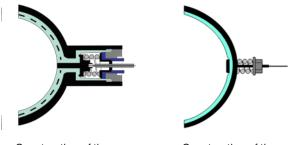
Construction of the electrode for PFA liner Construction of the electrode for PTFE liner
