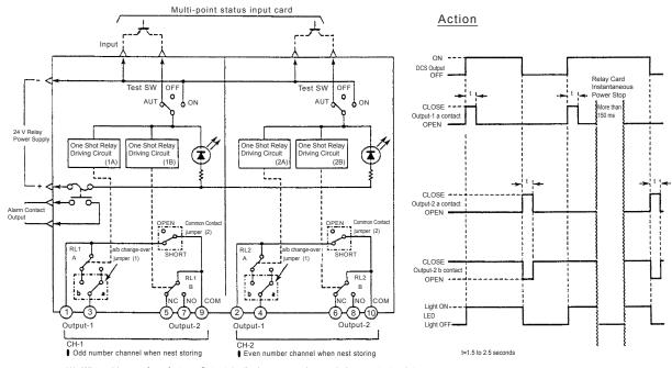
When shipment from factory, Output-1 a/b change-over jumper is in a contact point
