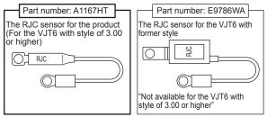
The style of VJT6 is indicated on the nameplate attached to the side face of the main unit.
