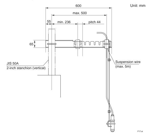
Jet Cleaning Unit for Free-standing Installation
