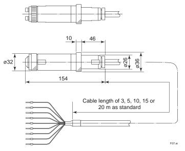
Note Air bubbles or dirt on the MLSS sensor can interfere with accurate measurement, especially in the low concentration level. For such applications, take an appropriate measure, e.g., tilt the sensor approximately 30° or add a cleaning system.
