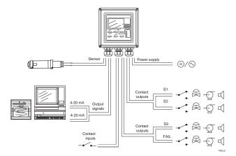
Figure 5 Example of External Wiring
