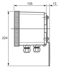
Panel Mounting Brackets (Option Code: /PM) Weight: approximately 0.4 kg
