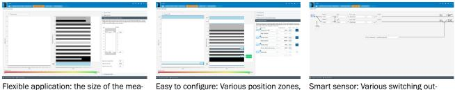
Flexible application: the size of the measuring range can be changed and adapted to the application conditions Easy to configure: Various position zones, thresholds or widths can be configured and monitored by means of different switching criteria Smart sensor: Various switching outputs and external inputs can be logically linked. This makes the sensor flexibly configurable for a wide variety of applications
