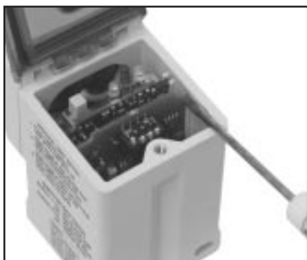
Figure 1. Remove the output card using a small screwdriver to dislodge it from its connector.
