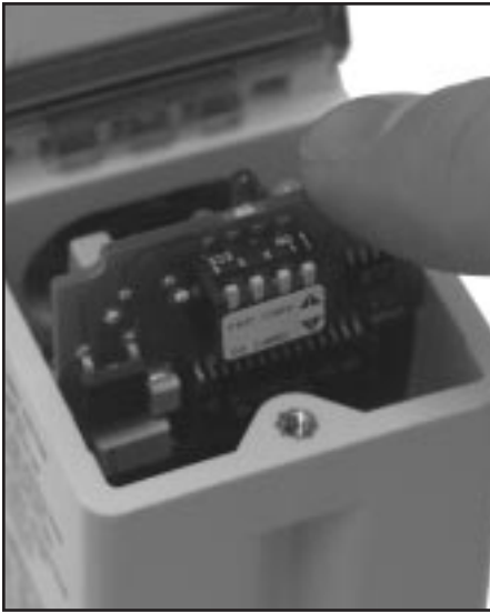
Figure 3. Slide the Q45UML card into the sensor and push it firmly into place.
