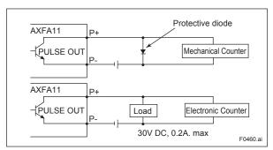
Figure 4.4.13 Pulse Output Connection
