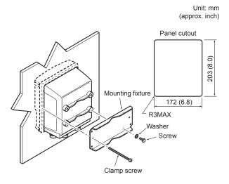
Fit the AXFA11 into the panel. Then attach the mounting fixture to the AXFA11 using the screw and the washer, and secure the instrument with the two clamp screws.
