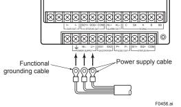
Figure 4.4.9 Electric Cable Wiring for AXFA11 Remote Converter
