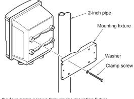
Pass the four clamp screws through the mounting fixture, position it on the 2-inch pipe, and then fasten the AXFA11 in place.
