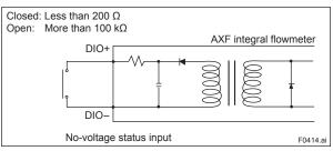
Figure 4.1.14 Status Input Connection
