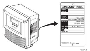
Figure 2.1.4 Name Plate (AXFA11 Remote Converter)
