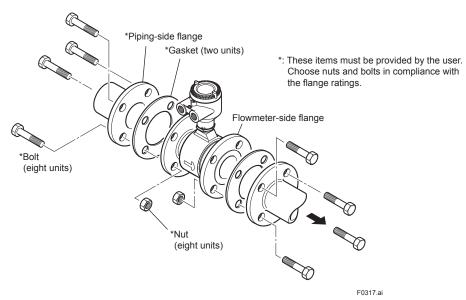
Figure 3.3.5 Mounting Procedure for Flange Type (sizes: 2.5 to 400 mm (0.1 to 16 in.))
