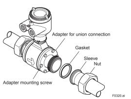
Figure 3.3.7 Mounting Procedure for Union Connection Type
