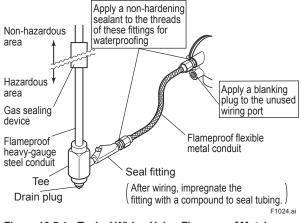
Figure 10.5.4 Typical Wiring Using Flameproof Metal Conduit
