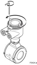
Figure 4.2.8 Removing the Terminal Box Cover for Remote Flowtube
