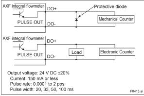
Figure 4.1.13 Active Pulse Output Connection (Optional code EM)
