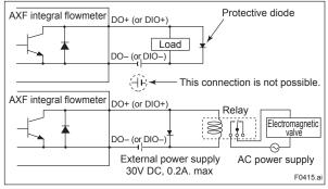
Figure 4.1.15 Status Output / Alarm Output Connection
