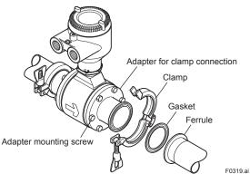
Figure 3.3.6 Mounting Procedure for Clamp Connection Type
