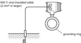
Class D requirements (grounding resistance, 100 Ω or less).
