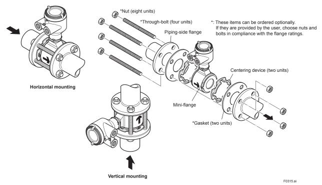
Figure 3.3.3 Mounting Procedure for Wafer Type (sizes: 25, 32 and 40 mm (1.0, 1.25 and 1.5 in.))
