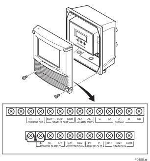
Figure 4.4.8 Terminal Configuration Labels position for AXFA11 Remote Converter
