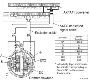
Figure 4.2.13 Wiring Diagram
