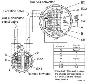
Figure 4.2.14 Wiring Diagram
