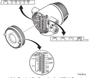
Figure 4.3.6 Terminal Configuration for AXFA14 Remote Converter
