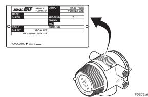
Figure 2.1.3 Name Plate (AXFA14 Remote Converter)
