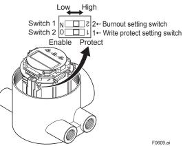
Figure 6.3.2 Switch Configuration for Integral Flowmeter and AXFA14 Remote Converter
