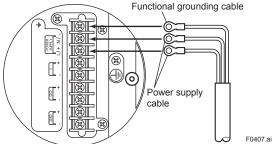
Figure 4.1.7 Electric Cable Wiring for Integral Flowmeter
