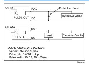
Figure 4.3.12 Active Pulse Output Connection (Optional code EM)
