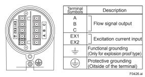
Figure 4.2.10 Terminal Configuration for Remote Flowtube (Explosion proof Type)
