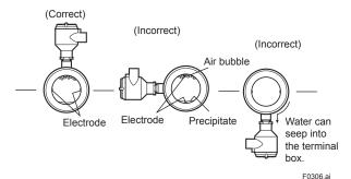
Figure 3.1.6 Mounting Orientation
