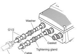
When working on conduit pipes or flexible pipes (G1/2 only) F0449.ai
