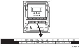
Figure 4.4.7 Terminal Configuration for AXFA11 Remote Converter
