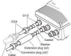
When working on electric wire tube or flexible tube (G3/4) \* When connecting G1/2, remove the conversion plug and connect directly to wiring port. F0451.a
