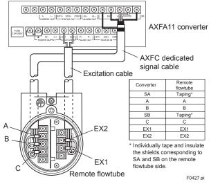
Figure 4.2.11 Wiring Diagram
