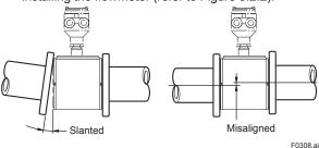
Figure 3.2.2 Slanted and Misaligned Flowmeter Piping
