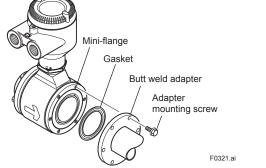
Figure 3.3.8 Mounting Procedure for Weld Joint Adapter Type
