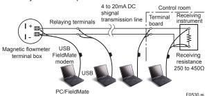
Figure 5.5.2 Connecting the HART Configuration Tool
