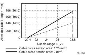
Figure 4.3.8 Supply Voltage and Cable Length for AXFA14 Remote Converter
