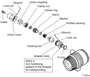
Figure 10.5.3 Installing Flameproof Packing Adapter
