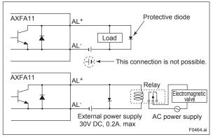
Figure 4.4.17 Alarm Output Connection
