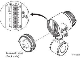
Figure 4.1.6 Terminal Configuration for Integral Flowmeter
