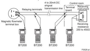
Figure 5.5.1 Connecting the BT200
