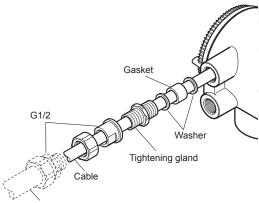
When working on conduit pipes or flexible pipes (G1/2 only) F0402.ai
