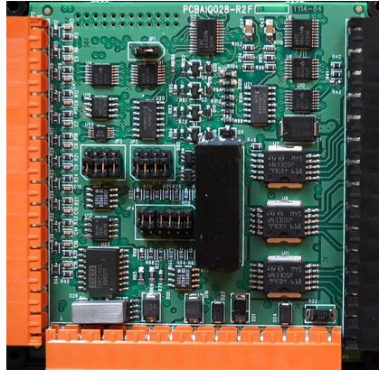
Figure 11.2 - XL4 I/O Cover Removed (sample I/O board)
