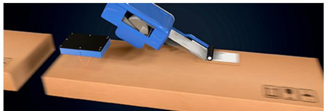
The SPEETEC detects positions on piece goods. As a result, it is possible to process piece goods at the right position.
