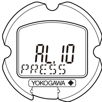
Self-diagnostic error on integral indicator (Faulty transmitter)
