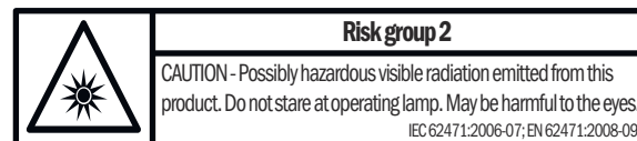
Figure 1: Risk Group 2: Caution - Possibly hazardous visible radiation emitted from this product. Do not look into the lamp during operation. This could damage your eyes.
