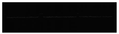
Figure 32: Too short exposure time: Laser line hardly visible.
