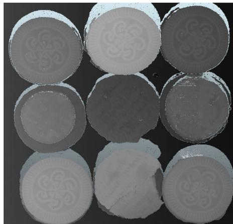
Figure 44: 3D image with range information as brightness.
