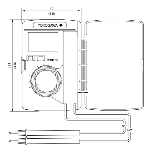
Thickness when the protection cover is closed: approx. 18mm (approx. 0.7 inch)
