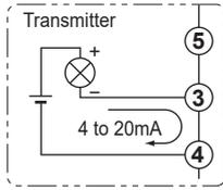
(1) Combination with two-wire type transmitter using internal power supply
