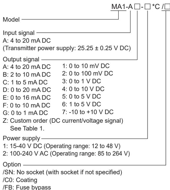
(Note 1) "/C0" option: Polyurethane coating. The "/C0" option does not guaranteed the coating effect though it is expected that the corrosion resistance for electric circuit is reinforced. And it is not able to submit coating test data.
